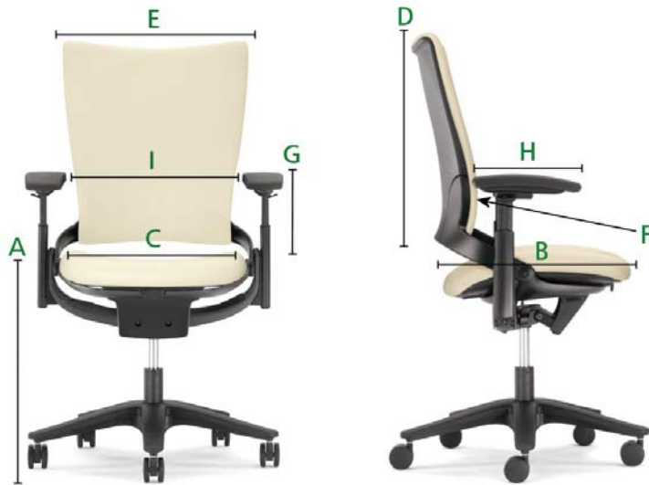
Figure 8. Measurements from BIFMA guidelines used for ergonomic chairs. See Table 3 for values. (Allsteel Sum™ task chair pictured)
